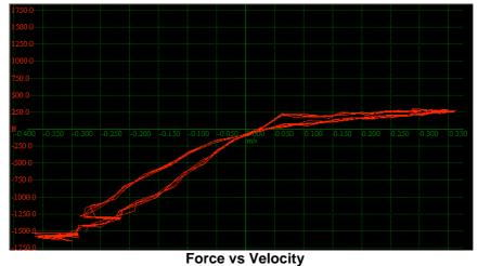
For positive speed (push) force is close-constant (flat), for negative speed force is proportional to speed.
