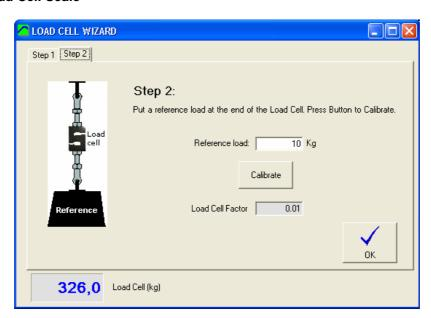
With the calibration weight pulling the load cell, enter the calibration weight value on the white box and press the "calibrate" button.
