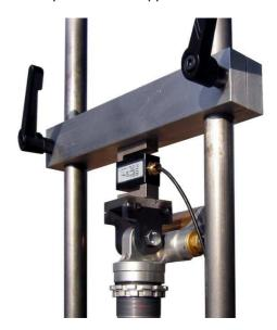
When adjusting the upper bar, the user should ensure that the shock absorber can move along all its displacement and it doesn't reach its boundaries because in such case, the force applied to load cell will be very high and it could be damaged.
