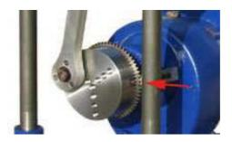
The sensor is thought to be placed horizontally in the machine (0 degrees) but if its position is different, it can be configured in the software: "sensor offset".
