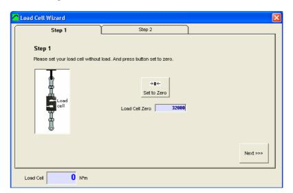
With the load cell free, press the "set to zero" button and check the "load cell zero" value is between 30000 and 35000, otherwise there may be some problem on the wiring.
